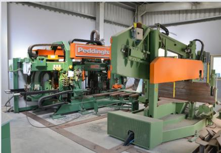
The Advantage-2 high-speed drill line in tandem with a structural band saw aid in increased production in Al Reyami's new facility.
