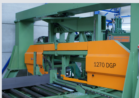
The Peddinghaus DGP saw and BDL-1250 provide the backbone for structural fabrication at Geerits.
