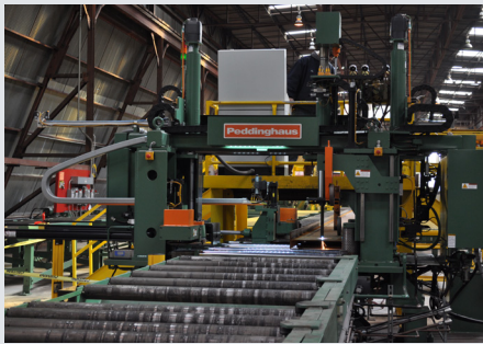
The three torches on the ABCM-1250 creates the fastest and most efficient copers on the market today.
