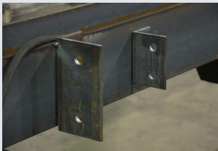
Detail components and beams leave the SBA fully fit-up and welded as dictated by the original design.
