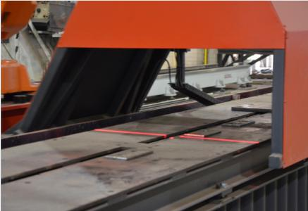
The machine scans parts to be welded to the main section.
