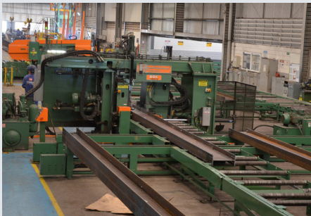
The all new BDL-1250/9D at Codeme is able to process upwards of 180 beams in single shift of hours.
