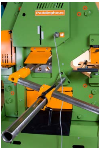
Universal electrical contact length stop, for 39 inch cutting length ref. no. 522.1
