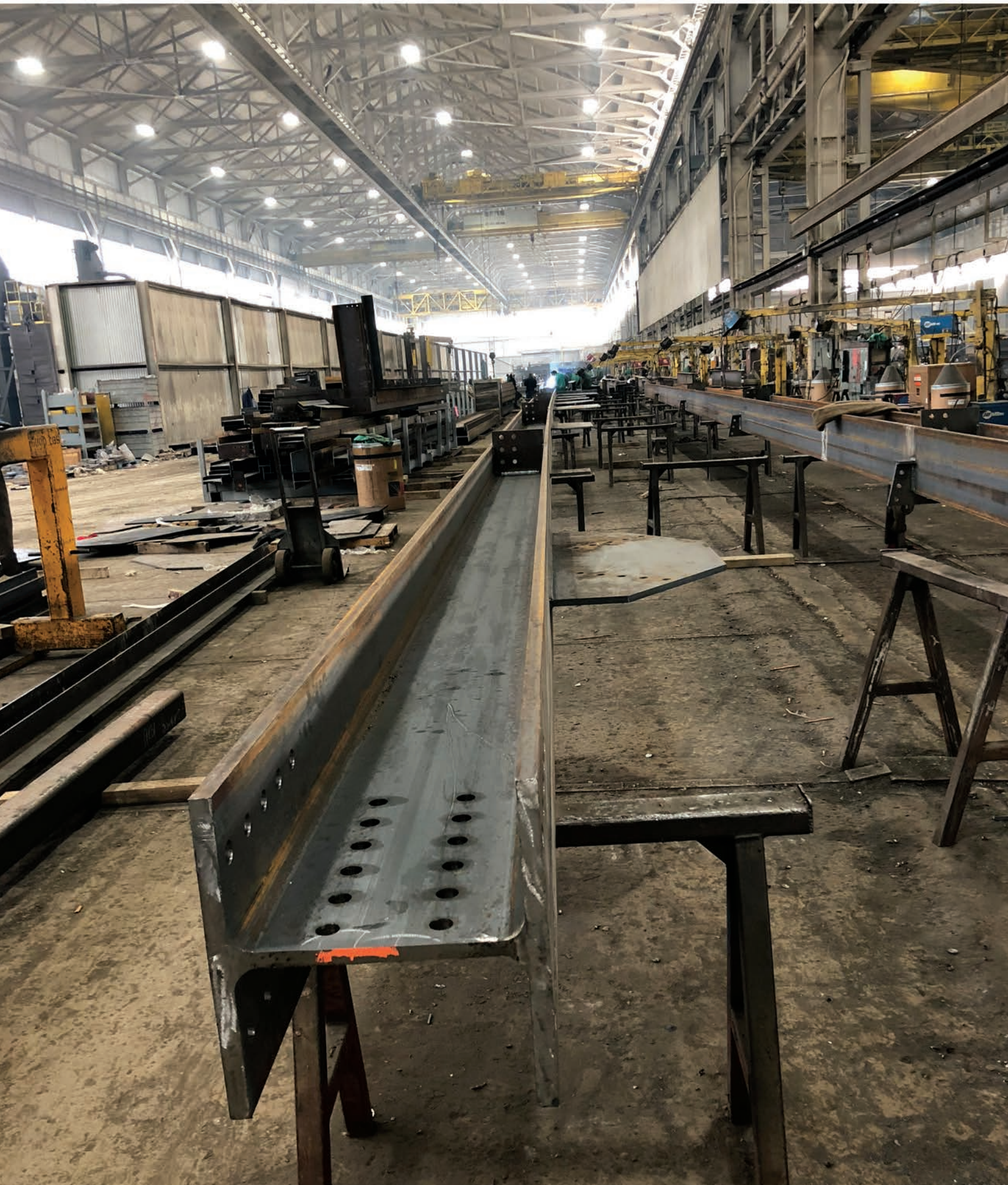
Sippel Steel located in Ambridge, Pennsylvania processed this massive 109 ft long beam on their Peddinghaus BDL-1250/9D drill line, with better than 1/16" accuracy.
